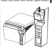
Open the cover with cover open button 2 Put a roll paper in the right direction
